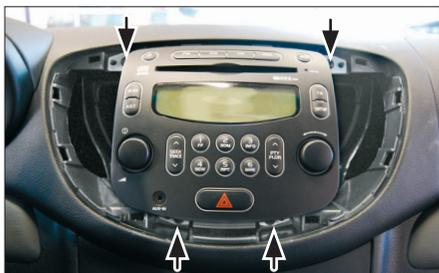
4. Remove the 4 screws (see arrows) fixing the OEM head unit
