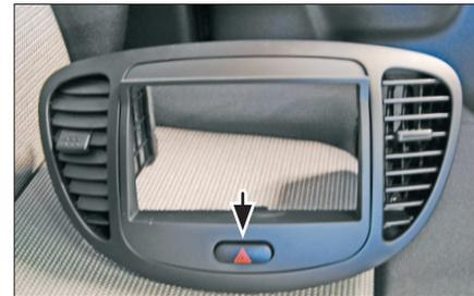
6. Center panel with installed hazard switch
