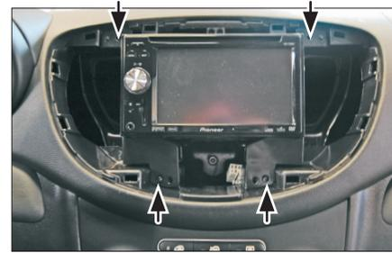
4. Mount the Double DIN Navigation to the Mounting Frame. Connect all required circuit points and place the Double DIN Navigation with the mounting frame on the dashboard. Fix it with the 4 original screws (see arrows)
