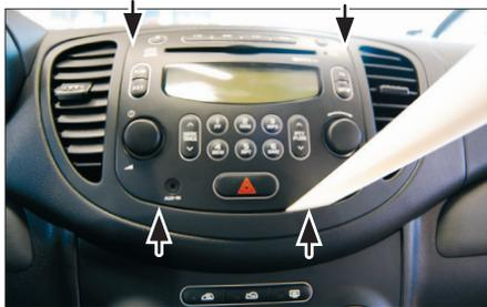
2. Unclip carefully the center panel surrounding the OEM head unit
